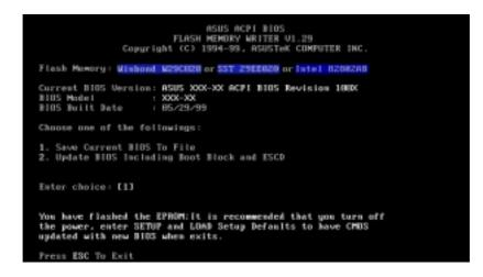
**WARNING!** If you encounter problems while updating the new BIOS, DO NOT turn off the system because this may cause boot problems. Just repeat the process, and if the problem still persists, load the original BIOS file you saved to the boot disk. If the Flash Memory Writer utility is not able to successfully update a complete BIOS file, the system may not boot. If this happens, call the ASUS service center for support.
