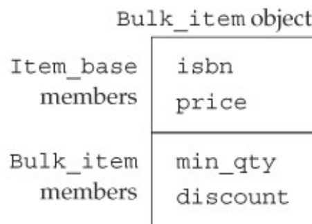
Figure 15.1. Conceptual Structure of a Bulk_item Object
