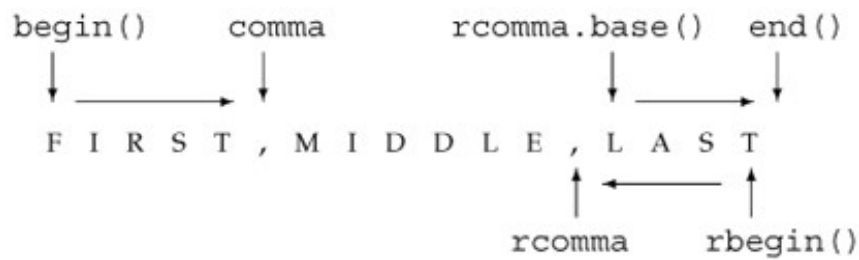
Figure 11.2. Relationship between Reverse and Ordinary Iterators
