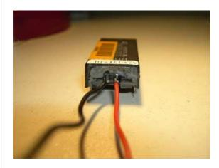
Then connect the wires to a battery pack equipped with a 3V-lithium cell:
