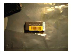
The next step was to remove the plastic of the cap and the unterlying resin at the site opposite to the little dot inicating pin 1 of the chip. I used a mini drill for the first 2 millimeters and after that a sharp blade to remove the filling from two "wires" or solder bumps located in the lower half of the chip:
