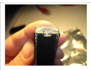
Now you'll have to carefully solder two wires to the solder bumps. Please note the polarity of the bumps. If not sure use a multimeter on the bumps to assure that you don't mix them up. The connector closest to pin 14 is ground (black), the pin closest to pin 15 is +3V (red).
