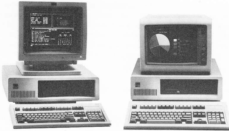
Two members of the IBM line of personal computers for which versions 1 and 2 of MS-DOS were developed. On the left, the original IBM PC (version 1.0 of MS-DOS); on the right, the IBM PC/XT (version 2.0).
